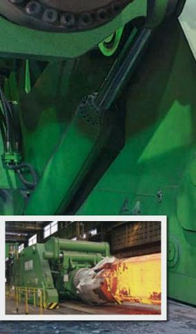
Rail-bound forging manipulators by DANGO & DIENENTHAL are equipped with high-dynamic drive systems. The machines are designed for use at high performance forging presses.
