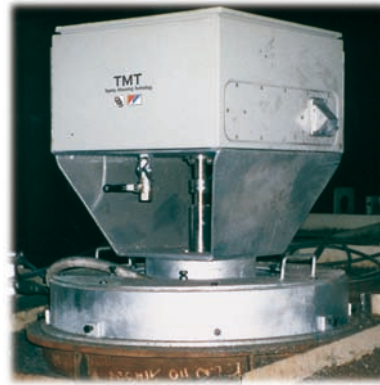
Radar electronics in a protective housing to suit steel work environments
