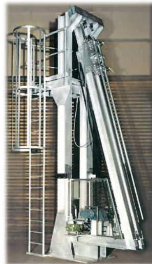
Iron Temperature and Sampling Lance
