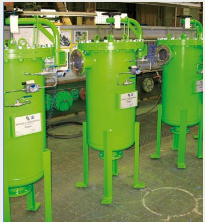
Fig. 5 Bag Filter in welded design
